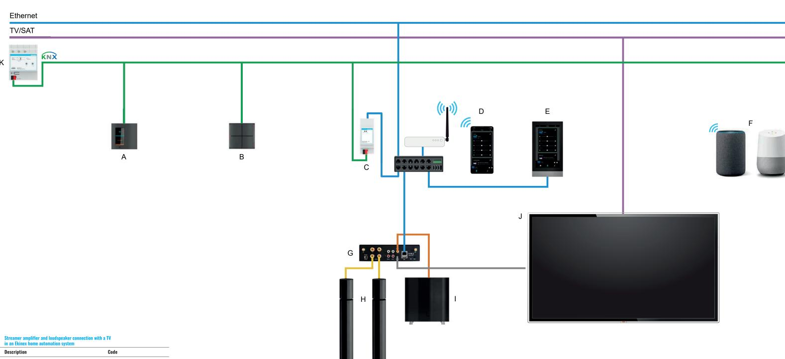
EK-EV3-TP a) Signum virtual button **b)** FF series wall-mount device EK-ED2-TP EK-DEL-SRV-BAS-200-TP **c)** Delégo Server d) App Sentio/Delégo for mobile devices e) Delégo panel 5" EK-DEL-5PAN o EK-DEL-5PAN-P f) Amazon Alexa - Google Home voice command support EK-50S-AU g) Streamer amplifier 50Wx2 EK-OMNI-... o EK-IRIDE-... h) Omni/Iride series speakers i) Subwoofer EK-K-... o EK-Q5-... o EK-Q6-.. j) TV (not supplied by Ekinex) **k)** BUS power supply EK-AB1-TP
